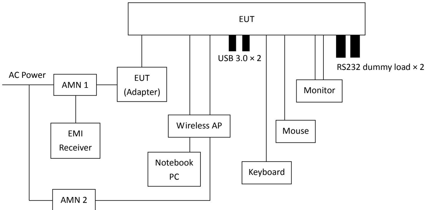
The EUT along with its peripherals were placed on a 1.0 meter(W) $\times$ 1.5meter(L) and 0.8 meter in height wooden table and the EUT was adjusted to maintain a 0.4meter space from a vertical reference plane. The EUT was connected to power mains through a Artificial Mains Network (AMN), which provided 50 ohm coupling impedance for measuring instrument and the chassis ground was bounded to the horizontal ground plane of shielded room.
